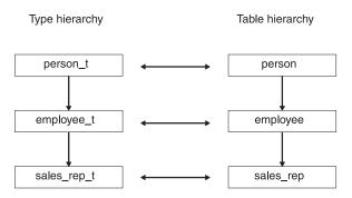
Figure 9-5. Example of the relationship between type hierarchy and table hierarchy
