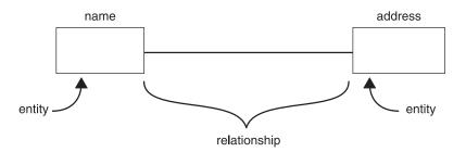
Figure 2-12. Symbols of an Entity-Relationship diagram
